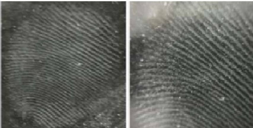
Figure 3. Fingermarks developed on glass surface with S(6/1). Right image shows the same marks but with slightly higher magnifications
